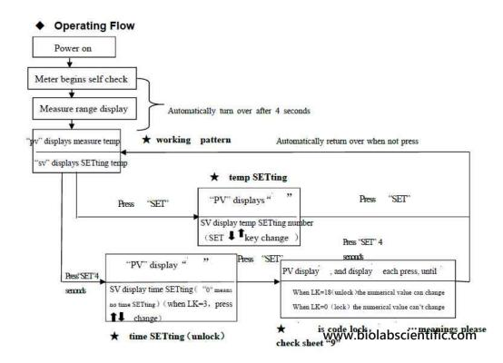
The modification of the temperature controlling parameters
